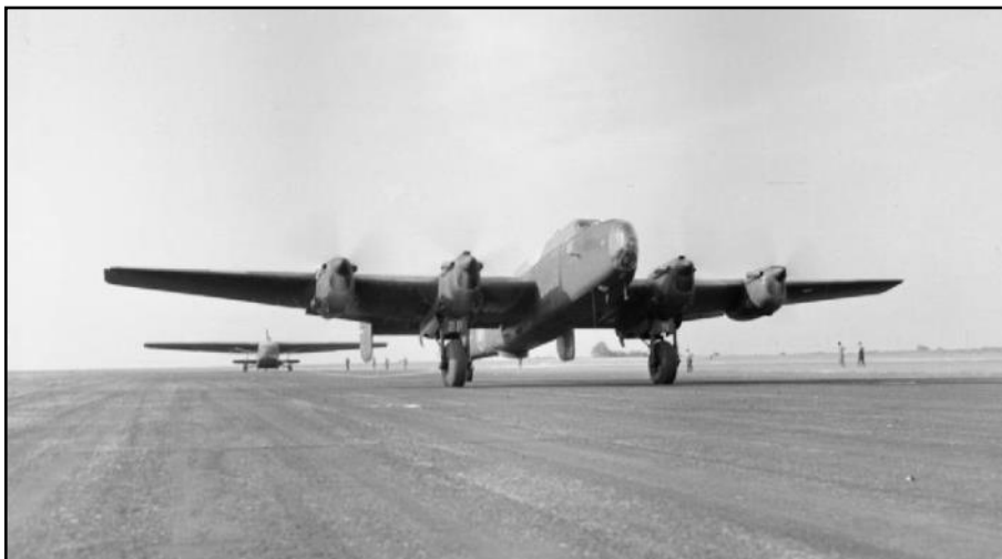
Merlin-engine Halifax MkV 1A LL218 of No 644 Sqn at RAF Tarrant Rushton with a Hamilcar glider in tow, prior to take-off.
